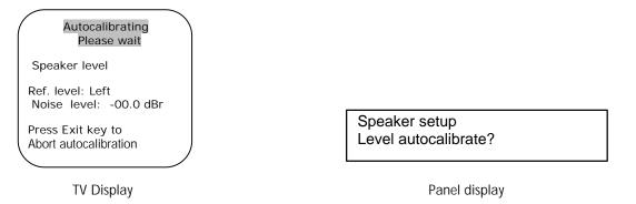
Pink noise (at a low level) will automatically begin from the left front speaker and rise slowly in volume. The SSP-60 generates this noise, listens through the microphone, then increases the signal level gradually until the Sound Pressure Level at the listening position is 75 dB. The SSP-60 will test every speaker in the same sequence as described above and set their levels to 75 dB.
